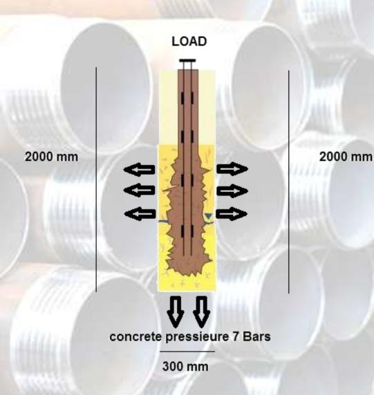
The Load is now applied at all circumference as well as the "head " of the micro pile. We are at this point getting a Load resistance equal to a 3m2 plate footing foundation for a 7" injected micro pile.
