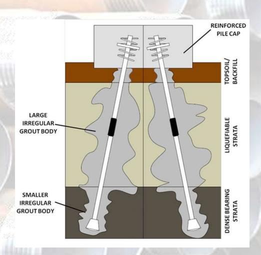
The particularity of our injected micro piles as it is injected under pressure, it will fill in every cracks, cavities and reinforce every liquefiable Strata
